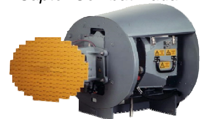
Grifo Mechanical Scan Combat Radar
